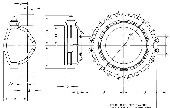
FOR INSTALLATION BETWEEN 125# OR 150# ASA FLANGES (18" & 20" ONLY, THESE FOUR HOLES ARE TAPPED "AB" X "AD" DEEP EACH FACE)
